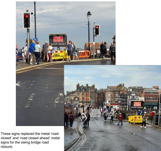
The traffic signals were configured to stay on 'all red' between the hours of 10:30 and 16:00 during road closures
